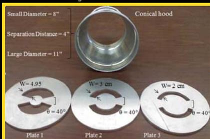
Figure 1: Design plates and the conical hood
