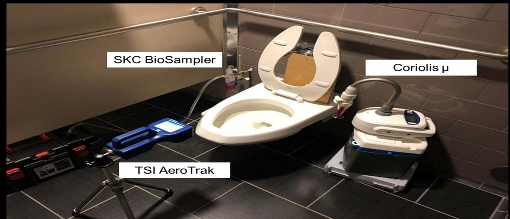
**Figure 1.** Sampling setup showing a SKC BioSampler (12.5 L/min) and Coriolis  $\mu$  sampler (150 L/min) containing Hank's Balanced Salt Solution placed 0.15 m away from the toilet to collect aerosolized MNV.
