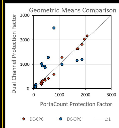
**Overall geometric mean protection factor measured with the dual channel instruments relative to that measured with the PortaCount**
