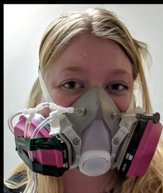
**Test subject donning the respirator.** The port on the subject's left is plugged while the port on the subject's right has two Y connectors for consistent sampling from inside the respirator.
